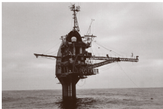
Fig. 18.38 R/P FLIP drifted freely so the hull rotated to remain in the same orientation to the prevailing wind
